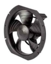
The EXRi50 series fan pack is a fully integrated assembly that has been aerodynamically designed to deliver high efficiency flow rates at static operating point 25 pascal (0.10 in-H2O) and below. It is suited to low power evaporator applications.
